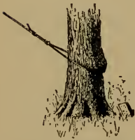
170. The wrong way of attaching a guy rope.
