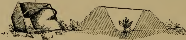
191. Forcing-hill, and the mold or frame for making it.
