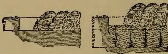
81. Trenching with a spade.
