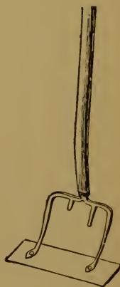
100. Home-made scarifier or scraper.
