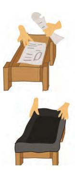
7. Cover the boards with newspaper to avoid damaging the plastic sheet with splints and nails. Place the plastic sheet in the container on top of the newspaper.
