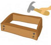
2. Nail the four boards together to form a frame. Put the 1.04 metre boards on the outside and the 1.00 m boards on the inside.
